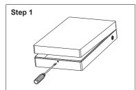
Remove the screws at the bottom of the unit. Lift up the Main Switch Knob and Power Knob to make it free. Remove the front plate gently.
